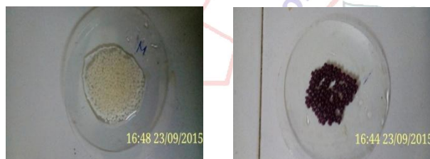
Fig. (1) A photograph showing the swollen (A) Alginate and (B) Gold encapsulated Alginate polymeric beads
