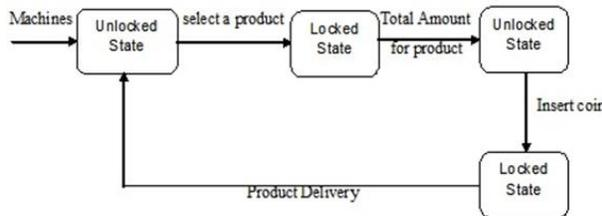
Fig. 4.2 Locked and Unlocked Transition
