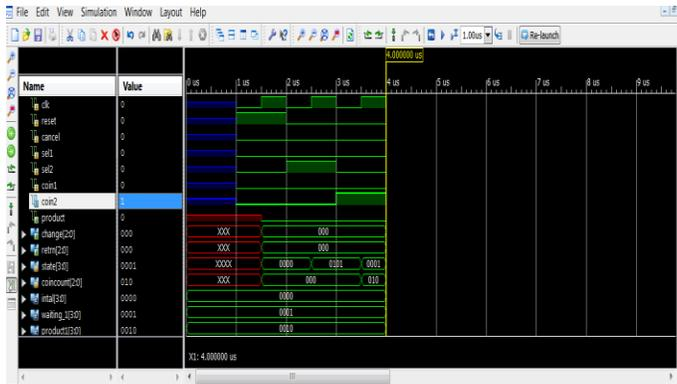
**Fig.5.1. Snapshot showing waveform in Mealy machine**
