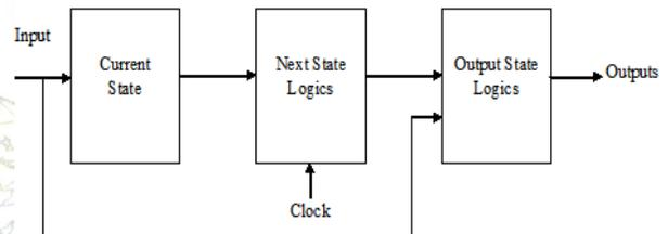
Fig. 1.2 General diagram of Mealy machine
