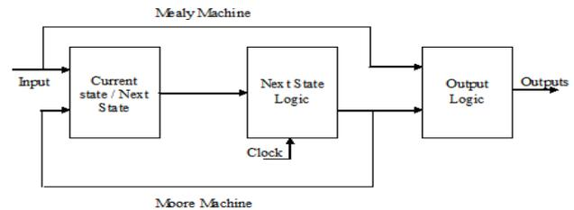
Fig. 1.1 General Structure of FSM
