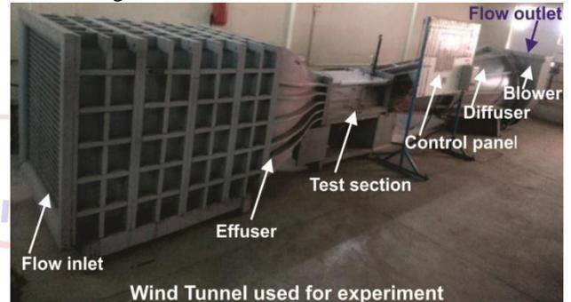
Fig.1.2 Wind tunnel used for the experiment at Christian college of Engineering and Technology, Bhilai. Different section of the tunnel as marked over the tunnel.
