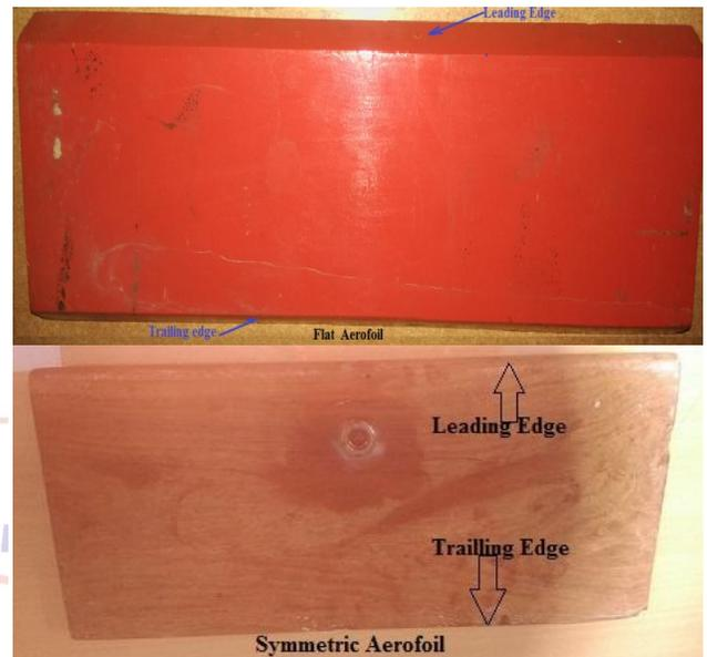
Fig.1.4 Shows the three different types of aerofoil has taken for experimental purposes, (a) Camberd, (b) Flat and (c) Symmetric aerofoil.
